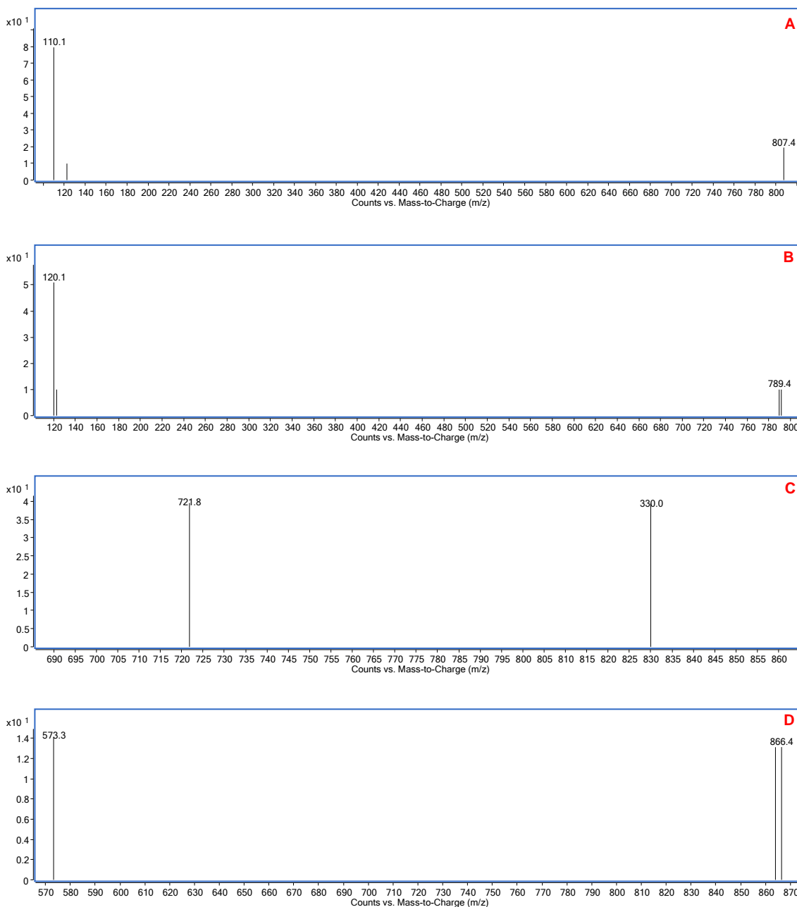
Figure 60: MRM spectra of Hb \beta^{93}\text{Cys} peptide modified by APAP (A-B), MDMA (B), and THC (D) obtained with the electrochemical trapping assay.
