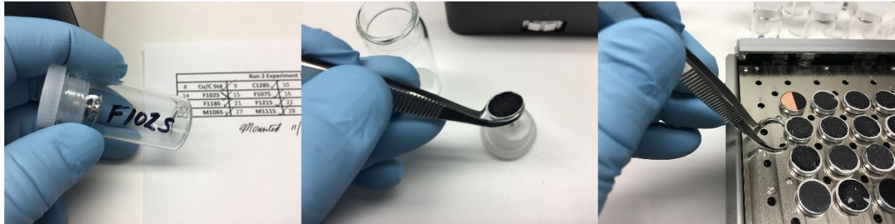
Figure 1. SEM stub in storage container (left), removal of stub (middle) and mounting of stub on the SEM sample holder (right).
