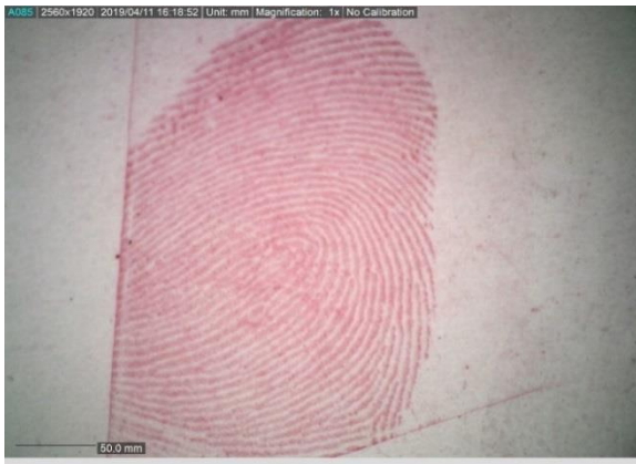
Figure 7. Fingerprint lifted by the traditional method from a paperweight using clear tape with red powder.
