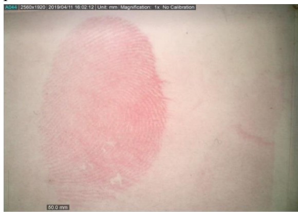
Figure 21. Fingerprint lifted by the traditional method from a mouse using clear tape with red powder.
