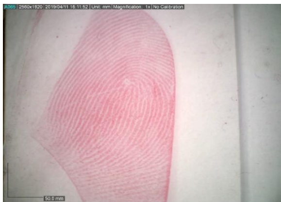
Figure 26. Fingerprint lifted by the traditional method from a cabinet handle using clear tape with red powder.
