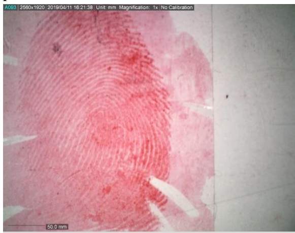
Figure 23. Fingerprint lifted by the traditional method from a doorknob using clear tape with red powder.
