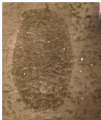
Figure 2. Fingerprint reverse-lifted from a mug using masking tape with adhesive-side developer.
