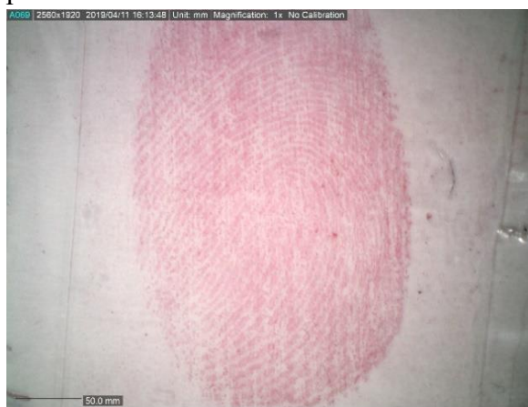
Figure 20. Fingerprint lifted by the traditional method from a door using clear tape with red powder.
