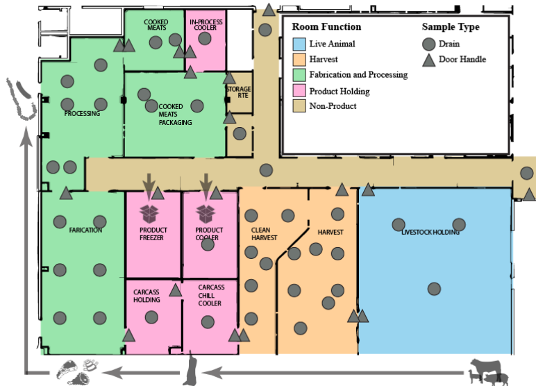
Figure 2.4. The GFIC facility layout and experimental design. Rooms within the facility are categorized by the general function. The sampling sites are identified by their location within the facility by either circles (drains) or triangles (door handles). The general flow through the facility is indicated by arrows and icons representing the product held in the spaces.
