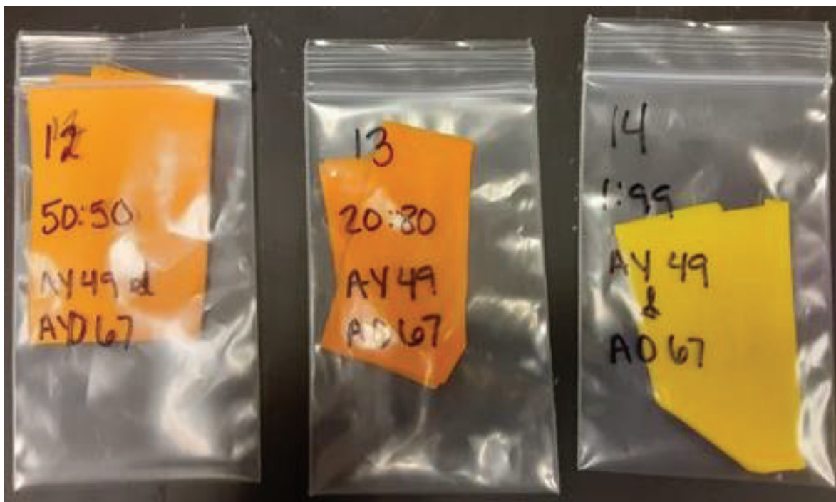
Figure 61. Fabrics prepared with different amounts of AY49 and AO67. The 50:50 dyed sample is very orange, becoming increasingly lighter as the orange concentration is decreased. When only 1% AO67 is used, the fabric becomes a vibrant yellow.
