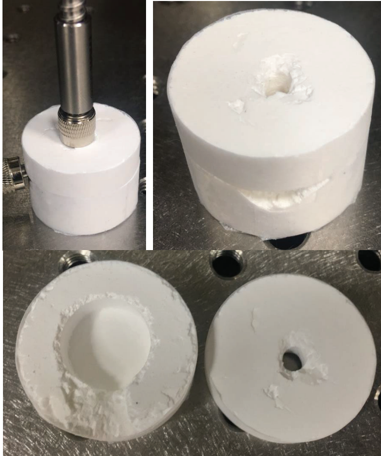
Figure 17. Aerosil OX 50 cavity w/5wt% binder with attached optical fiber. Without sintering, this material is very brittle and tends to crumble.
