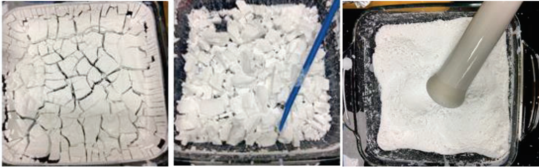
Figure 24. Crushing and grinding Aerosil OX 50 following incorporation of 5% binder.
