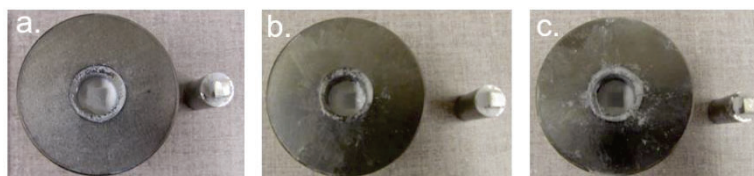
Figure 8. Aerosil powder pressed at various pressures for 5 min to yield a part with a cavity: (a) 500 lb, (b) 1000 lb, and (c) 2000 lb.
