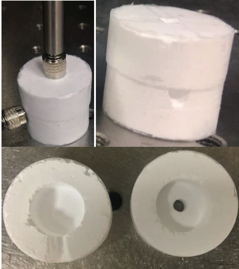
Figure 18. Aerosil OX 50 cavity w/5wt% binder, sintered at 1050 °C for 1 hr, with attached optical fiber. The sintered material is more stable and easier to machine.
