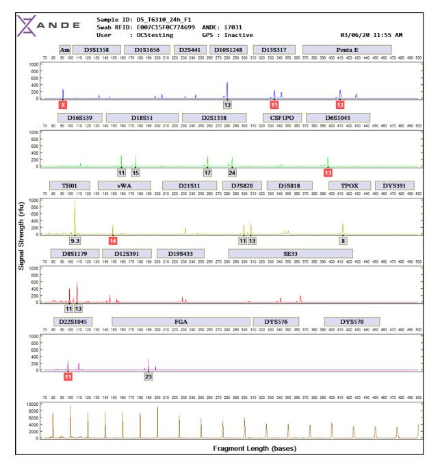
**Figure 2:** Example partial ANDE® profile. All alleles observed are correct, the grey alleles were automatically exported into an allele table and XML. The allele calls at D13S317, PentaE, vWA, D22S1045, and FGA include one of two expected alleles based on the donor's truth profile.
