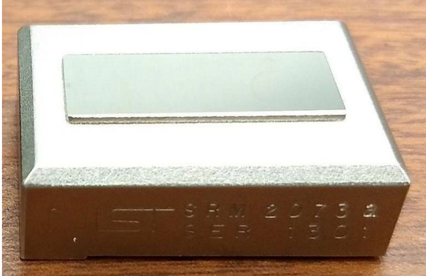
Figure 23 – NIST SRM 2073a sinusoidal roughness specimen
